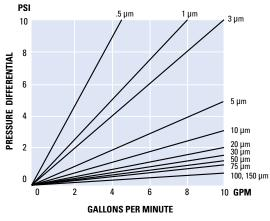
This chart represents the typical flow rate of polypropylene media per 10° cartridge length. The test fluid is water at ambient temperature. Extrapolations for multiple lengths tend to be linear, but as flows increase the differential pressure across the housing becomes more apparent.
