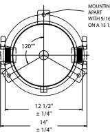
MOUNTING LEGS (3) 120° APART WITH 9/16" DIA. HOLES ON A 13 1/16" B.C.
