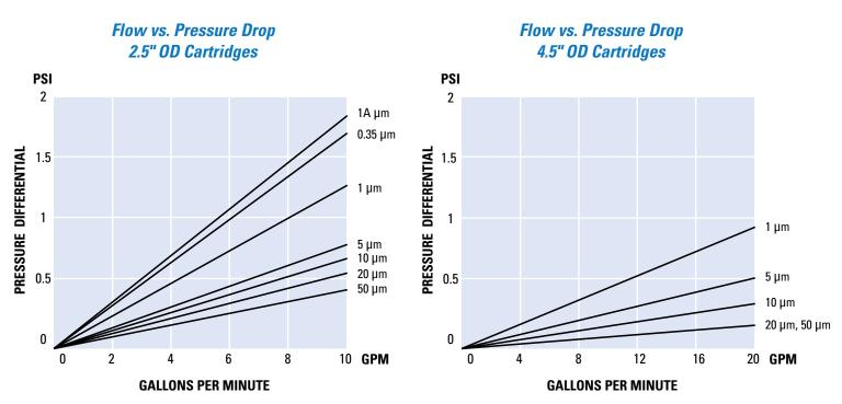
This chart represents the typical flow rate per 10" cartridge length. The test fluid is water at ambient temperature. Extrapolations for multiple lengths tend to be linear, but as flows increase the differential pressure across the housing becomes more apparent.
